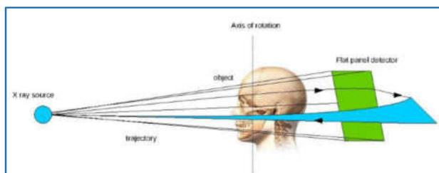
**Figure 1. Schematic Representation of the working Mechanism of a CBCT Scan unit**
