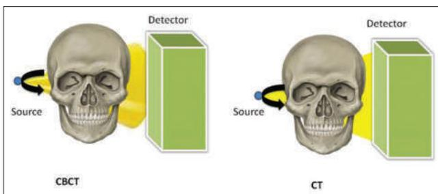
**Figure 1:** Comparison of the geometric configuration of incident X-ray beam projection and detector for cone-beam computed tomography and multidetector computed tomography
